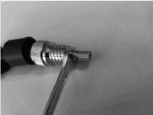
⑤ Remove the tip adapter using a 12mm wrench.
